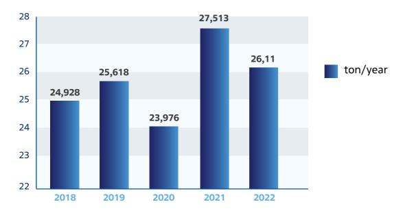
The reduction in pollutant emissions into the atmosphere was due to the uninterrupted operation of the refrigeration equipment in the chemical shop throughout the reporting period, as a result no unavoidable losses of refrigerant during opening, emptying and filling of freon vessels occurred.
